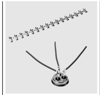
This terminal is used to connect a cluster pin (2.3mm in diameter) to a lead of a motor hermetically sealed in a compressor of a refrigerator, freezer or air conditioner. The contact is made of tin plated phosphor bronze to ensure a highly reliable connection for an extended period.
