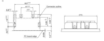
Note: 1. The above figure is the figure viewed from the connector mounting side.
