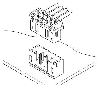
This 2.0 mm pitch insulation displacement connector is another version of the NRD connector for printed circuit boards. The KRD connector allows daisy chaining and is very useful in simplifying connection systems in electronic equipment.
