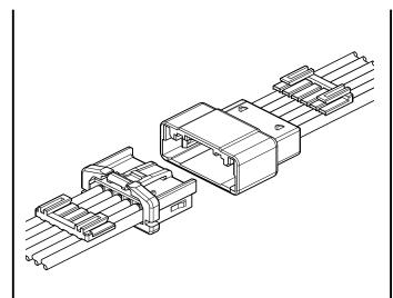
This connector is a 2.5 mm pitch wire-towire connector, having incomplete mating prevention mechanism. 2-circuit and 3-circuit connectors have control key to prevent connector from mating with incorrect circuits, thus, several same circuit connectors can be used.
